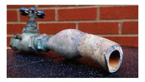
Image of a lead service line. Source: Associated Press.
