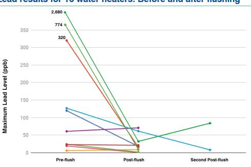
FIGURE 14 Lead results for 10 water heaters: Before and after flushing
